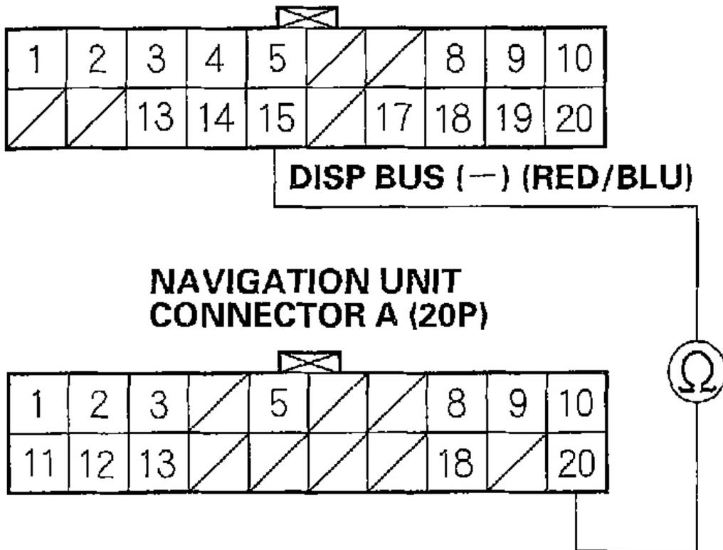
**Fig. 48: Checking For Continuity Between Display Unit 20P Connector Terminal No. 15 And Navigation Unit Connector A (20P) Terminal No. 20**
