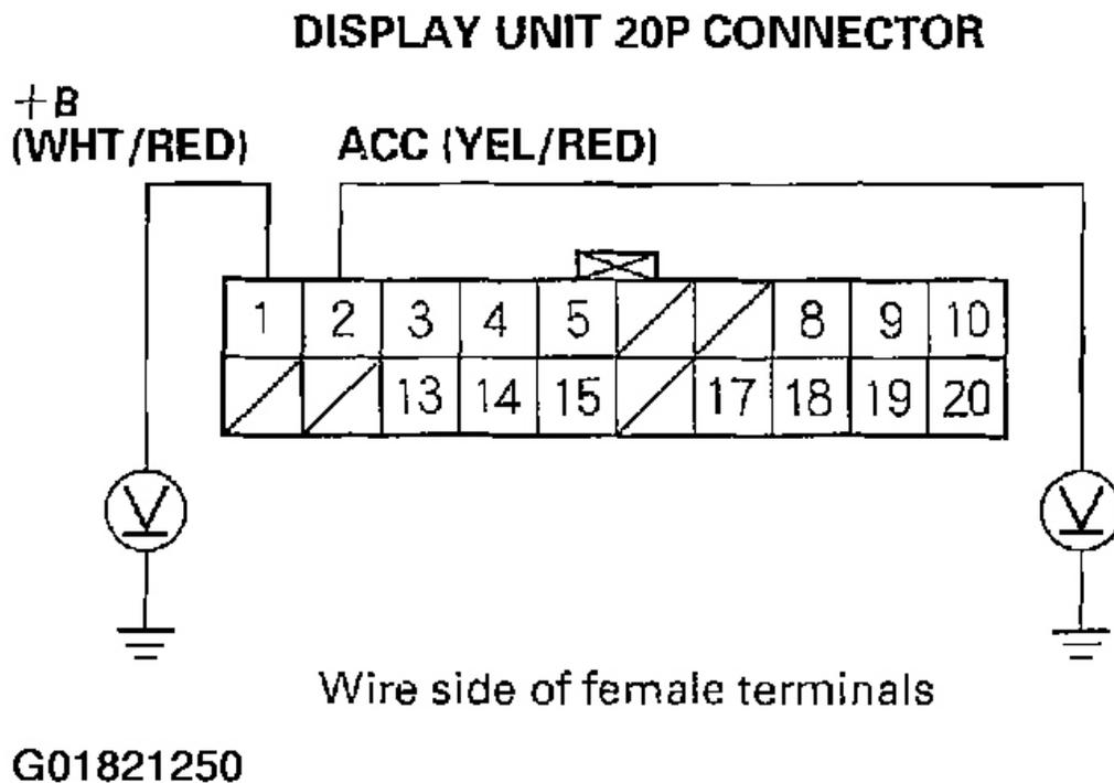
**Fig. 42: Measuring The Voltage Between Body Ground And Display Unit 20P Connector Terminal No. 1 And No. 2**
