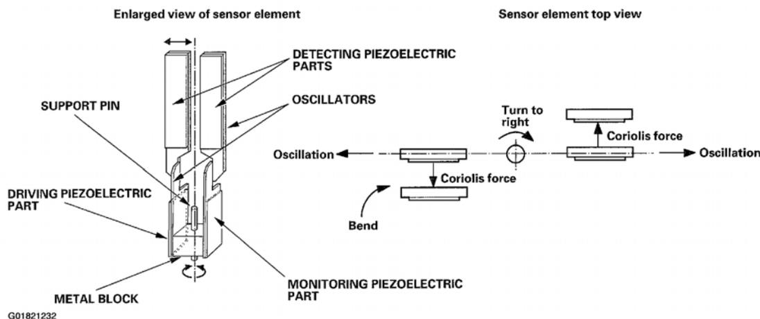
**Fig. 24: Piezoelectric Operation**
