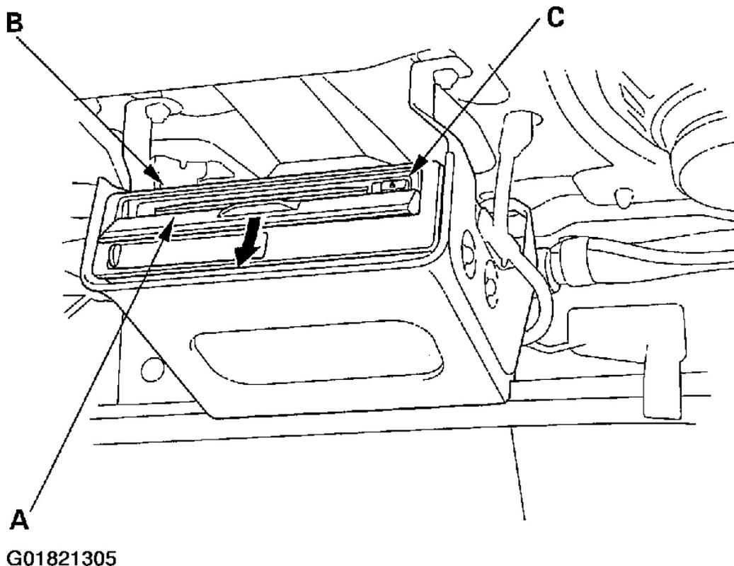
**Fig. 97: Opening The Front Cover Of The Navigation Unit Located Trunk Room**
